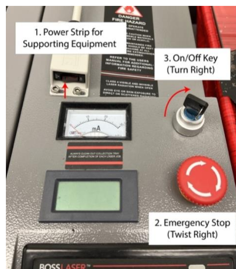
Figure 2. On/Off sequence for supporting equipment (1), releasing the emergency stop (2), and turning on the laser (3).
