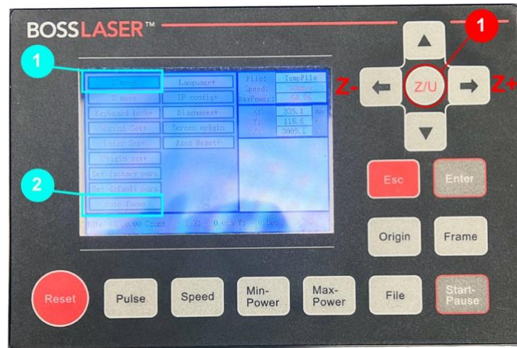
Figure 5. After pressing Z/U, menu options for moving the Z-axis (1) and autofocusing
