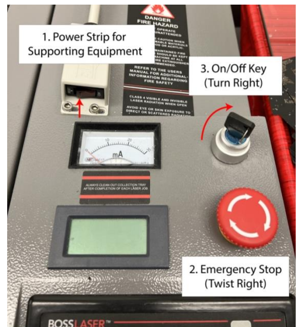
Figure 2. On/Off sequence for supporting equipment (1), releasing the emergency stop (2), and turning on the laser (3).
